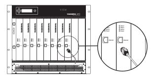
Connect a LAN cable from the Ethernet socket of the board just installed and to your network.
